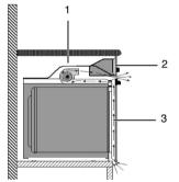
The built-in cooling fan cools both the built-in cabinet and the front of the appliance.
