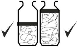
**IMPORTANT ALWAYS USE THE SPIN TUB DISC COVER AS THIS PREVENTS CLOTHING FROM RISING OUT OF THE SPIN TUB**
