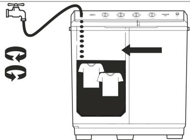
**6** OPEN THE TAP AND FILL THE WASH TUB WITH WATER TO THE DESIRED LEVEL, THEN CLOSE THE TAP
