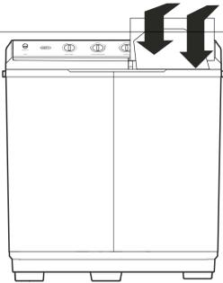
**3** CLOSE BOTH THE INNER AND OUTER LIDS OF THE SPIN TUB
