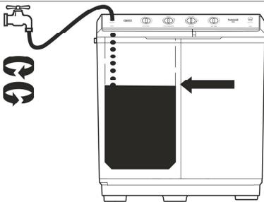
**5** OPEN THE TAP AND FILL THE WASH TUB WITH WATER TO THE DESIRED WATER LEVEL, THEN CLOSE THE TAP
