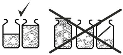
**2** PUSH THE WASHING DOWN GENTLY INTO THE SPIN DRUM AND PLACE THE DISC COVER IN THE DRUM SO THAT IT COMPLETELY COVERS THE WASH LOAD
