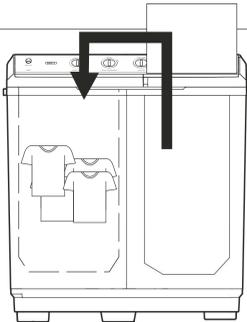
**5** REMOVE THE WASH LOAD FROM THE SPIN DRUM AND PLACE IT IN THE EMPTY WASH TUB
