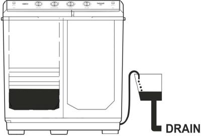
Front view of the washing machine with the drain hose connected to a drain. The drain hose is labeled 'DRAIN'.
