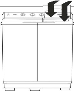
**4** CLOSE BOTH THE INNER AND OUTER LIDS OF THE SPIN TUB
