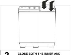
CLOSE BOTH THE INNER AND OUTER LIDS OF THE SPIN TUB
