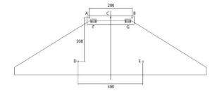
Screw the Outer Chimney to Plate I by screwing 2pcs of 4X8mm screws through the mounting holes at the top of Outer Chimney as shown in the following diagram.
