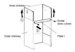
Screw the Inner Chimney to Plate II by screwing 2pcs of 4X8mm screws through the mounting holes at the top of Outer Chimney as shown in below diagram.
