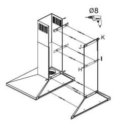
8). Screw the external chimney to the casing with 2 of the supplied 4X8mm screws.
